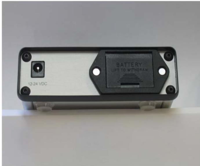
**12/24 VDC:** Plug the 12V charger into this port to charge the internal 9V rechargeable battery.
